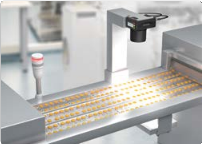
Blister pack inspection using BLOB Tool
