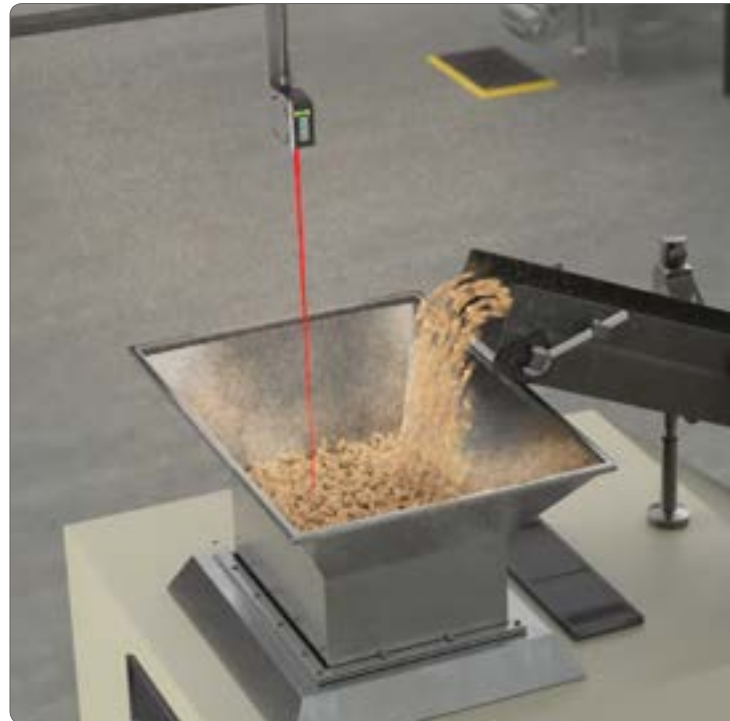
Monitoring levels inside a high-volume hopper
