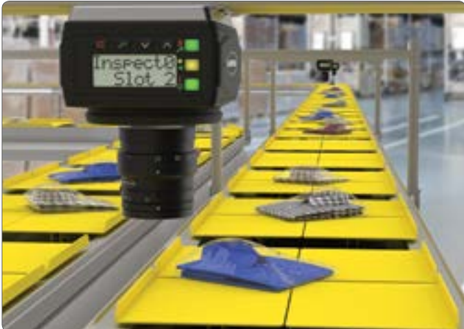
Empty sortation conveyor inspection using Blemish Tool
